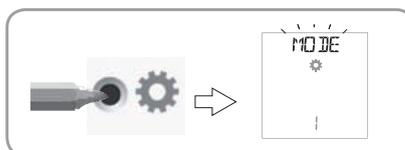
MODE <> RADIO <> SOLAR MOTOR <> SOFT <> RESET <> EXIT <> MODE ...
